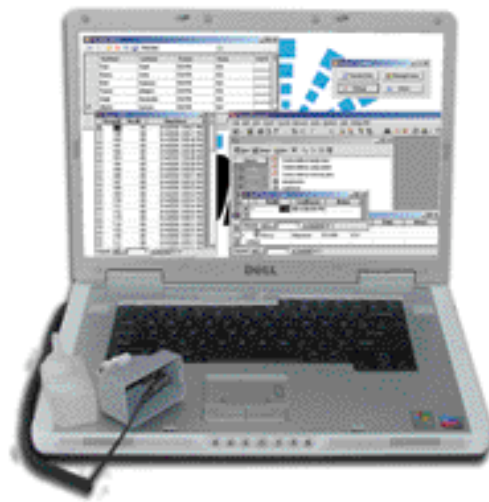
Personal sanitizer dispenser with tracking electronics downloading individual adherence data.
